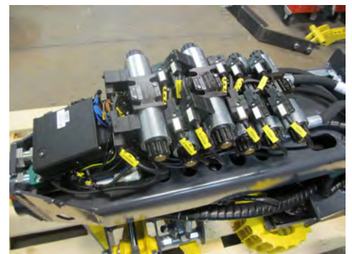
Valve board with CAN-slave module. All valves have diodes indicating functions.
