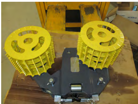
Roller package which can be retrofit. Well protected hoses.
