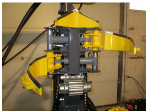
All knives are moving. Measuring wheel with magnetic pick-up.
