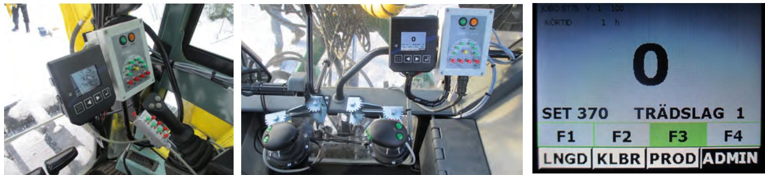
Excavator mounting with separate box for control buttons.
