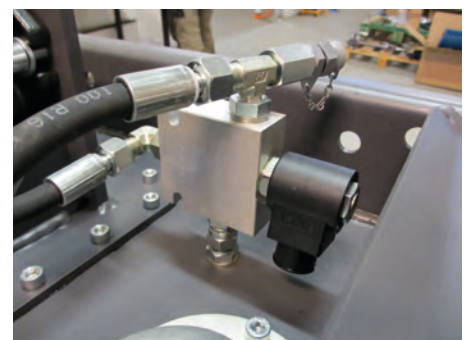
El. LS control for the pump. For crane LS-control an additional change over valve is installed.
