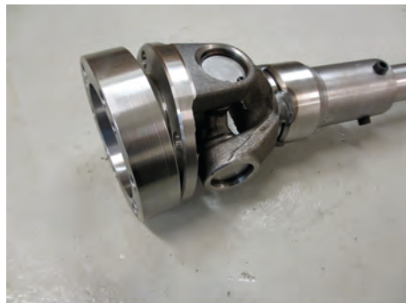
Drive shaft coupled to the crank shaft via cardan joint. Flexible jaw coupling on the pump.
