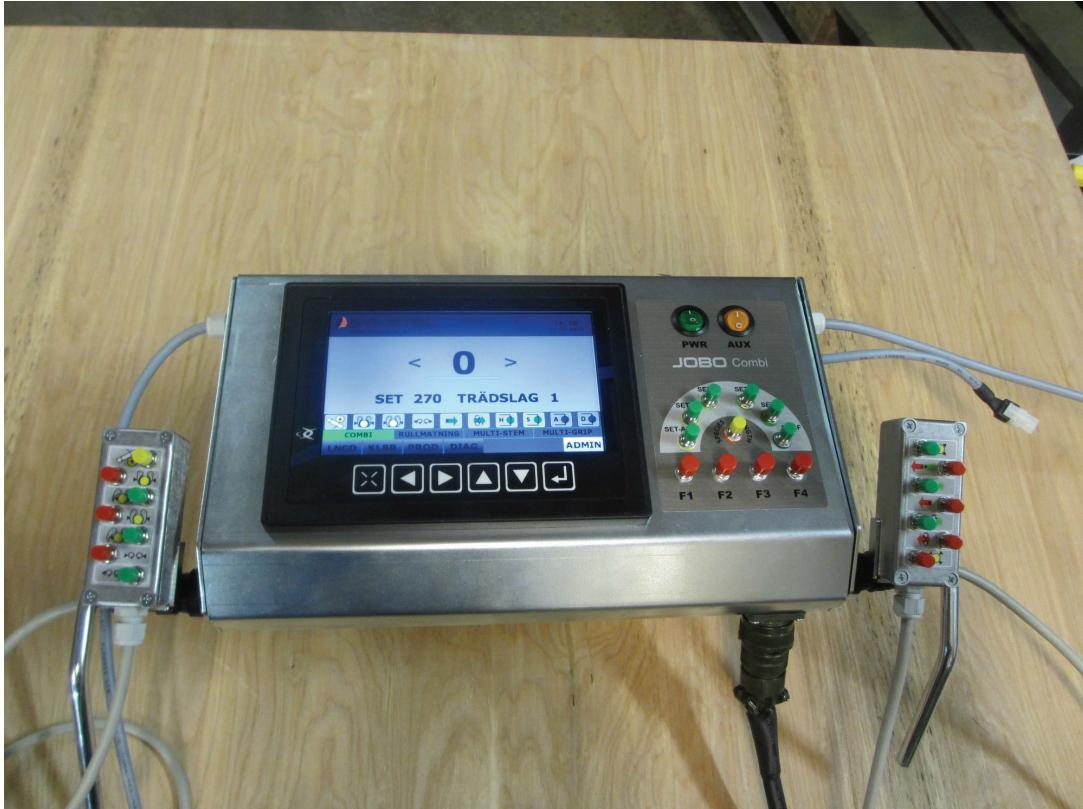
JOBO CAN MID is the more advanced measuring and control system built on high quality hardware with sophisticated features. The operating system Linux provides calculation power and easy to use menus to adjust all functions and even follow-up of produced volumes.
